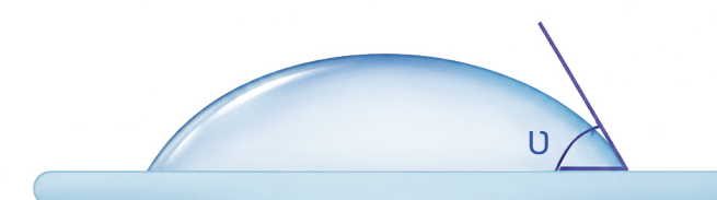
Non siliconized surface: U < 90^\circ
