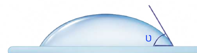
Non siliconized surface: U < 90^\circ
