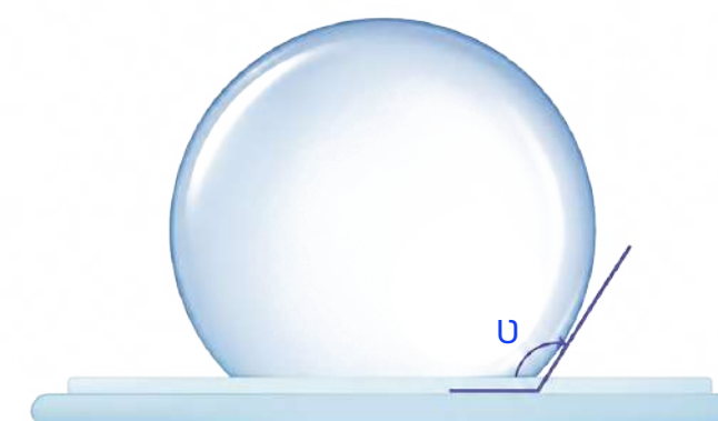
Siliconized surface: U > 95^\circ
