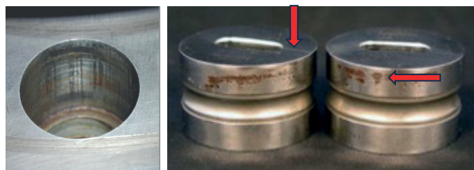
ABOVE: Fig 9 - Worn/damaged die pocket ABOVE RIGHT: Fig 10 - Fretted and cracked dies RIGHT: Fig 11 - Damaged die lock screw with contaminated threads
