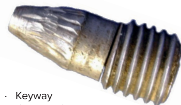
ABOVE: Fig 9 - Worn/damaged die pocket ABOVE RIGHT: Fig 10 - Fretted and cracked dies RIGHT: Fig 11 - Damaged die lock screw with contaminated threads
