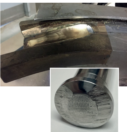
ABOVE: Fig 5 - Worn ejection cam INSET: Fig 6 - Severe ejection cam wear BELOW: Fig 7 - Worn die pockets from improper installation
