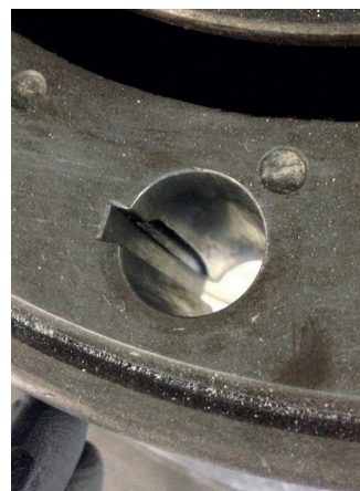
ABOVE: Fig 12 - Damaged keyway
